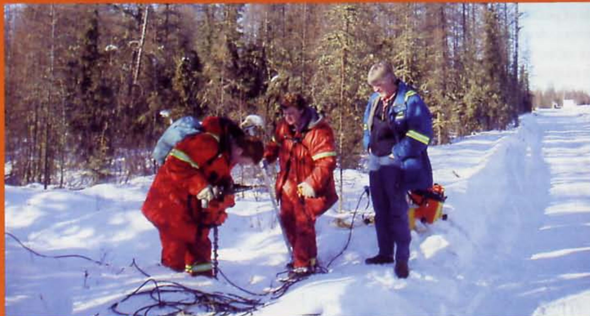
IMPROVING THE IMAGE A crew prepares a System Four VectorSeis Cable recording system for seismic acquisition in Alberta last winter. The "full wave" Input/Output system was brought to Canada by Trace Energy Services under contract to Apache Corporation.
